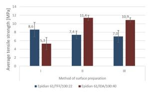
Fig. 4. The bonded joints shear tensile strength of 1.4310 sheets
