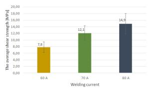
Fig. 3. The welded joints on shear strength of 1.4310 acid-resistant steel sheets
